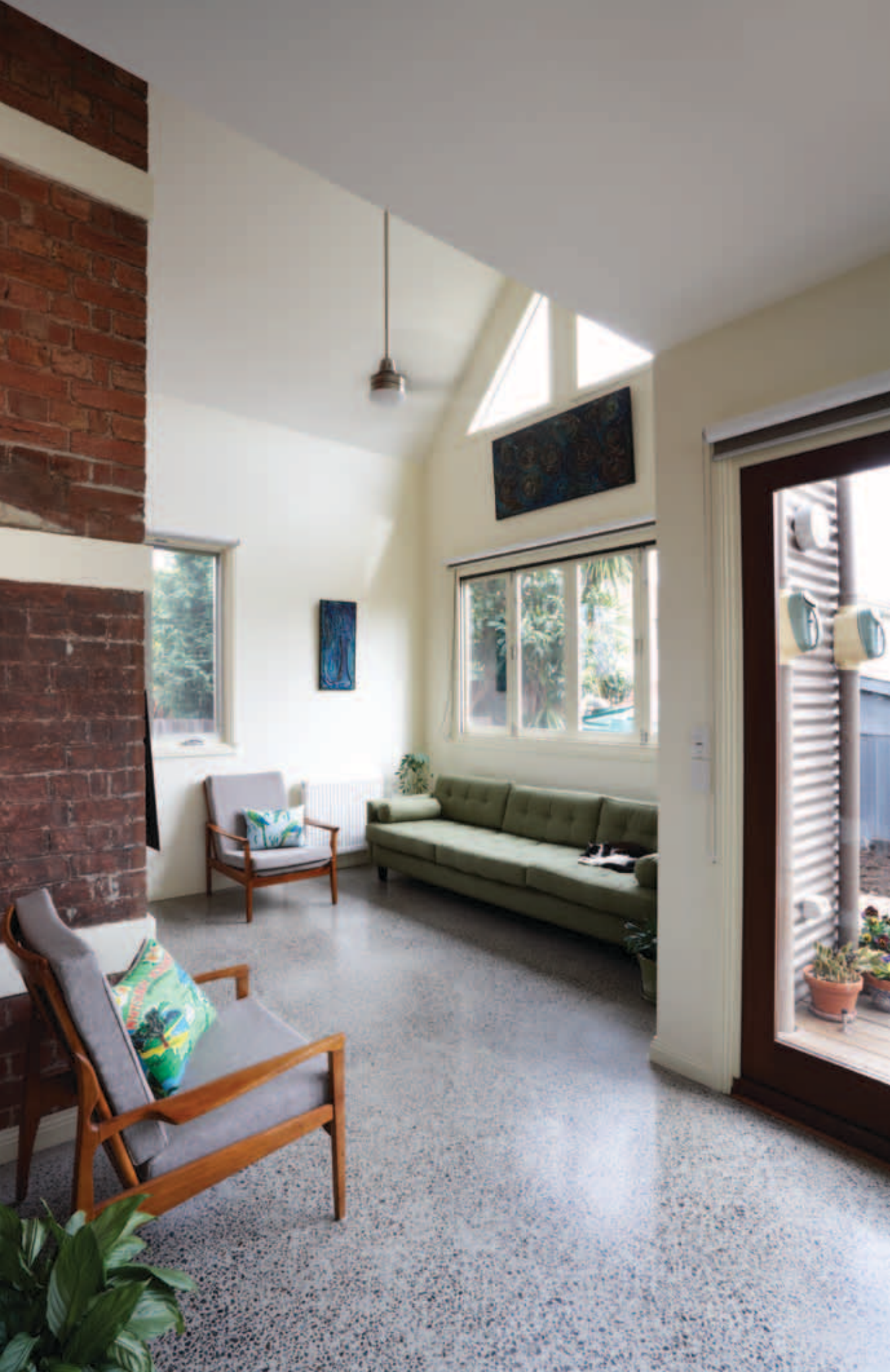
↻ Staying true to a philosophy of embracing the existing, the designers made a feature of the original external brick wall of the house, repainting the detail and incorporating it into the design of the living room. It also acts as thermal mass when low winter sun passes through the clerestory windows set high in the ceiling.
