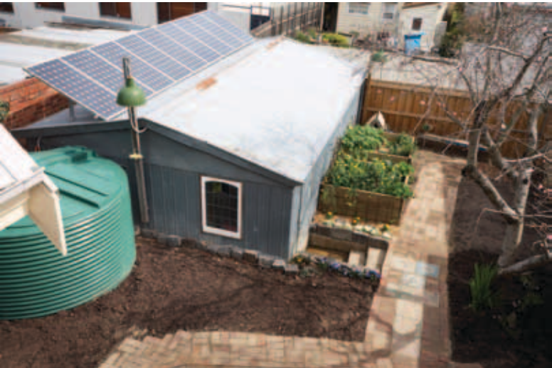
↺ From the roof terrace, views over the backyard illustrate some of the more obvious elements of the green renovation: the tank and photovoltaics. The rear fencing is Outdoor Timber Tanalised-E H3 pine treated with an arsenic-free preservative ( www.OutdoorTimber.com.au ). The posts for the fence are reclaimed cypress from Golden Cypress Rescued Timbers ( www.goldencypress.com.au ).
