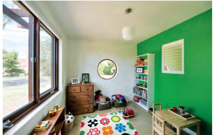
↑ The house’s orientation and layout bring sun deep within all living spaces. Louvred openings in internal walls aid the passage of cross breezes for ventilation and cooling.
