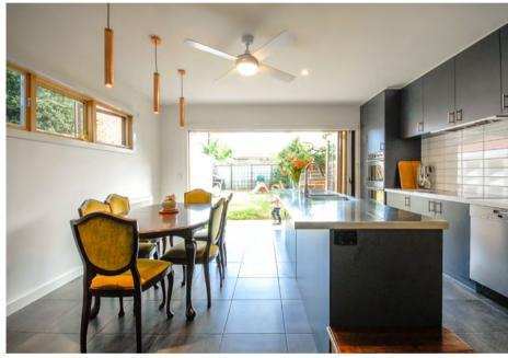
James and Jasmine opted for Australian-made tiles on their concrete slab floor, as it was a cheaper option than polished concrete and they were advised that the tiles wouldn't significantly impede the floor's thermal mass benefit.
